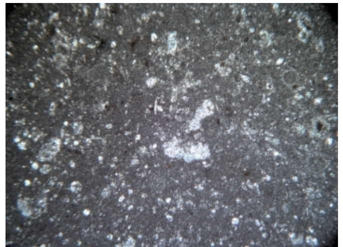
Figure 16a. / Figure 16b. Photomicrographs of diagenetic chert, formed by silicification of limestone sediments. Silicified planktonic foraminifera and a very few radiolarians are visible in the microcrystalline quartz matrix. A) Plane-polarized light. B) Crossed polars.
